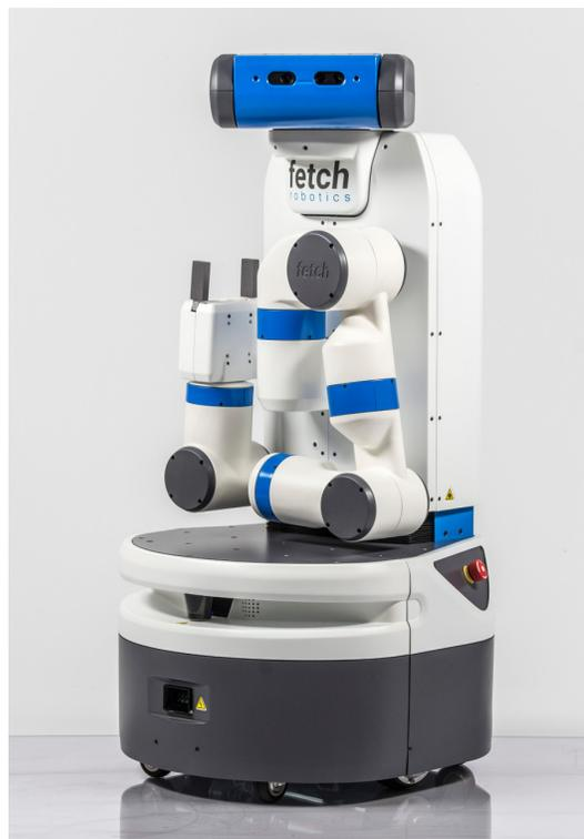
Fig. 1. The Fetch mobile manipulator for which this calibration system was initially designed. The robot comprises a 7-degree of freedom arm, pan and tilt head, torso lift joint, and RGB-D depth camera which must all be calibrated.
